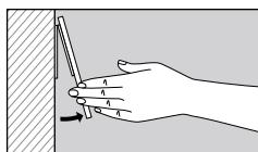
To make small adjustments to the planking, carefully lift the bottom of the plank, pulling up and away to expose the separated fasteners. Do not pull straight off. Adjust the position of the plank, then push the plank back onto the fasteners and push at each strip until you hear it click.
