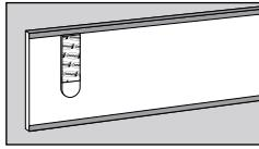
Remove one green liner from the pair and firmly press onto the backside of the plank. Repeat, applying pairs of strips to both ends of the plank and in the middle if over 2.5 feet.
