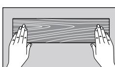
Remove the remaining green liners and press the plank directly onto the wall surface. Press firmly for 30 seconds, applying pressure at each strip to ensure adequate adhesive contact.
