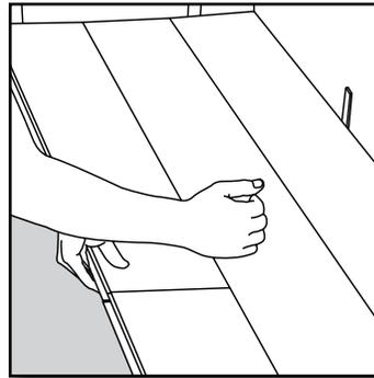
**[6]** If you wish to remove the flooring, just lift the planks a few inches and tap along the joint.
