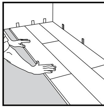
**[12]** The distance to the walls can be adjusted when three rows are completed. Remember to place the flooring a minimum of 1/4" from all walls or other vertical obstructions such as cabinets, pipes, or columns.
