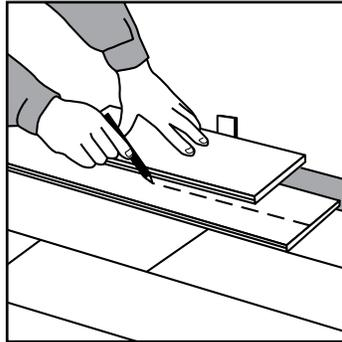
**[14]** Use a full width scrap plank and 1/4" spacer to mark your cutting line on the last row.
