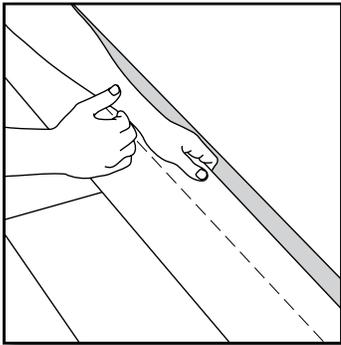
**[4]** Now remove the first row. Lift the planks a few inches and tap along the joint. Cut the planks as required.
