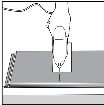
**[8]** Place the plank face down on the work surface and cut to size with a power saw. If you are using a hand saw, use a fine-toothed blade, and cut the planks face up.
