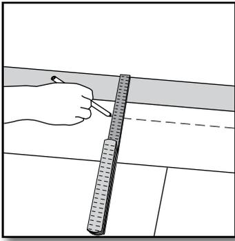
**[3]** If the starting wall is uneven, the planks must be adapted to its contours. You can scribe the contour of the wall onto the first row of planks using a 2" square block and a pencil following along the contour of the wall. Do not forget to allow for the minimum 1/4" expansion space from the wall. Disassemble the first row, cut the planks along the line you have drawn, and then reassemble. You will still use the spacers to maintain the expansion space along this wall.
