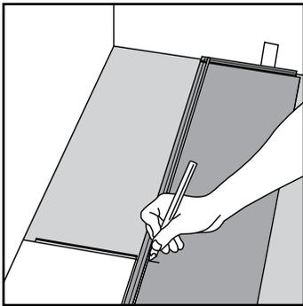
**[7]** Place the final plank face down with the short side (without the locking strip) towards the wall. The remaining expansion space should be at least a minimum of 1/4" from the wall. Draw a pencil line where the plank is to be cut.
