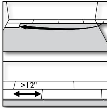
**[9]** Use a cut piece of board from the previous row to start the next row. This starting plank section must be at least 12" long. If the piece is too short, start with a new board. Cut the new board in one third, one half or two thirds length sections, depending upon what is required to maintain the random stagger from one row to the next. Always ensure that the end joints are staggered at least 12 to 16 inches from one row to the next.
