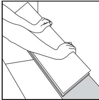
**[5]** Replace the first row by inserting planks from left to right. Press the first board with the groove toward the edge of the planks that are already in position.
