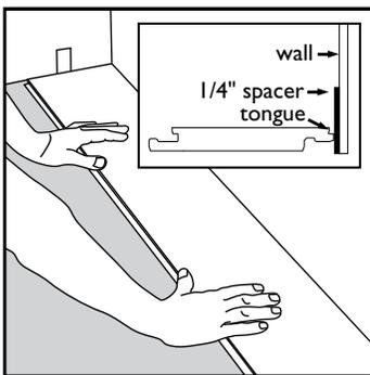
**[1]** Begin the installation in the left-hand corner against the wall. Place the plank a minimum of 1/4" from the left wall. Use the installation spacers throughout all perimeter areas to insure the correct expansion space is maintained.
