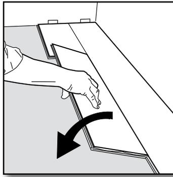
**[11]** Connect the planks in the following rows by aligning the end seam of each plank directly above the end seam of the preceding plank. Insert the long side seam at a slight angle first, and as the top surfaces meet, rotate the plank down into the locked position.
