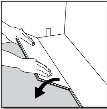
**[10]** Place the plank at an angle against the plank in the previous row. Press the edge forward against the previous row, and then fold down at the same time.
