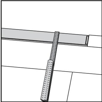
**[13]** Measure and cut the planks in the last row to fit. Remember to allow for a minimum of 1/4" expansion space from the wall.
