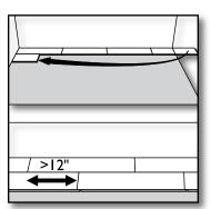
**191** Use a cut piece of board from the previous row to start the next row. This starting plank section must be at least 12" long. If the piece is too short, start with a new board. Cut the new board in one third, one half or two thirds length sections, depending upon what is required to maintain the random stagger from one row to the next. Always ensure that the end joints are staggered at least 12 to 16 inches from one row to the next.
