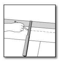
[3] If the starting wall is uneven, the planks must be adapted to its contours. You can scribe the contour of the wall onto the first row of planks using a 2" square block and a pencil following along the contour of the wall. Do not forget to allow for the minimum 1/4" expansion space from the wall. Disassemble the first row, cut the planks along the line you have drawn, and then reassemble. You will still use the spacers to maintain the expansion space along this wall.
