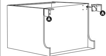
3. Place vanity in the desired position. Level the vanity, and shim under the faux legs (A) if necessary. Secure the vanity to the wall (refer to vanity installation instructions). Once leveled, place the inside of the side mouldings (B) against the sides of the cabinet with the bottom of the floor and the rear of the side moulding (B) touching the wall.
