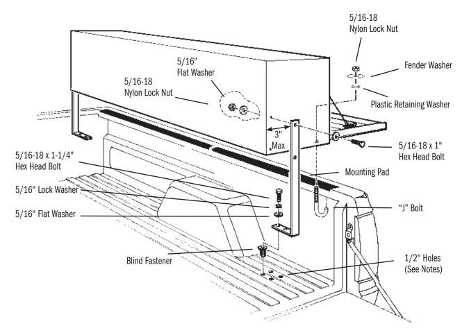
Place the mounting pads in position on top of the truck bed as shown in figure below. Tape the mounting pads to the truck bed in a few places to keep them from moving or falling off when installing the box.
