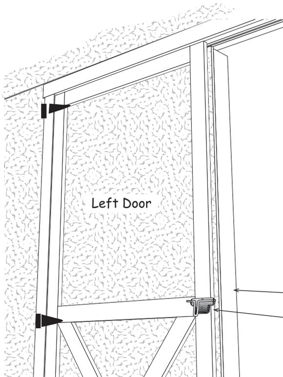
4. Before you fasten the hinges to the door trim, temporarily prop the doors in the opening. Set the door on a piece of OSB, see detail below. Leave a space at the top of the doors and between the doors and the side trim to allow room for the doors to expand when they absorb moisture.
