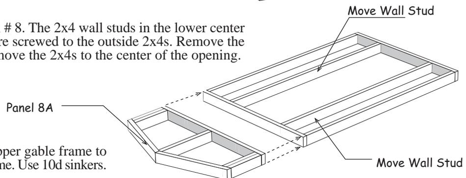
3. Install the upper gable frame to the lower frame. Use 10d sinkers.
