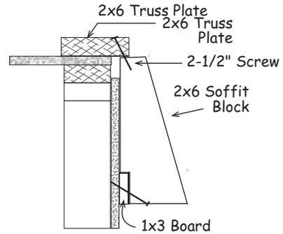
3. Position the 2x6 soffit blocks between the 1x3 board and the 2x6 truss plate. Secure the top of the soffit blocks in place by screwing through the 2x6 truss plate into the soffit block. Secure the bottom by toenailing through the bottom of the 2x6 soffit block into the 1x3 board. Use 7d coated nails. Install the soffit overhang on the opposite side of the building.
