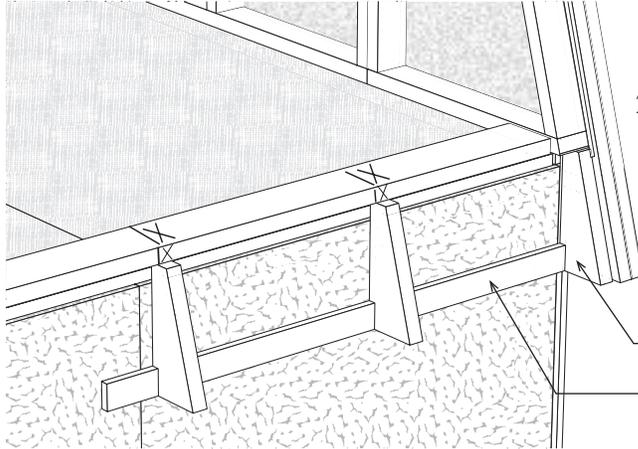
1. Extend the lines on the face of the 2x6 to the edge of the 2x6.
