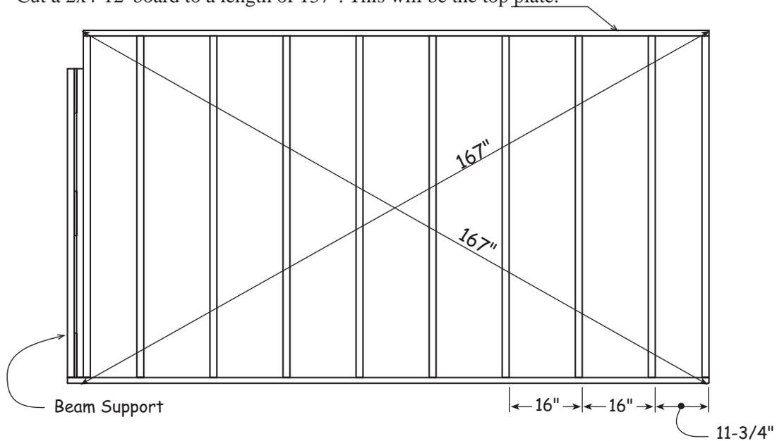
3. Install 92-5/8" wall studs between the top and bottom plates. Install the first stud 11-3/4" from the right end. Nail the treated bottom plate to the wall studs with 16d galv. deck nails. Use 16d sinkers to nail the top plate.
