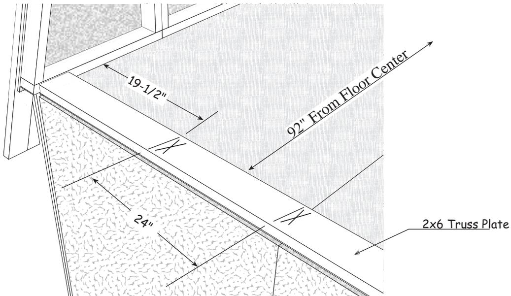
4. Layout 2x6 plate for trusses. **Important:** Start the truss layout 19-1/2" from the back of the gable plate. Then space trusses 24".
