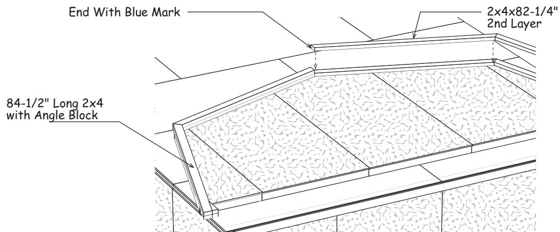
4. Locate (4) four 2x4s that are 84-1/2" long and have an angle block attached to one end. Install these 2x4s along the sides of the gable frame, extending 1/2" beyond the gable frame.
