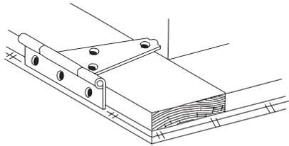
1. Lay the left door with the trim facing up. The 2x4 frame on the left door extends past the door trim. See detail below.
