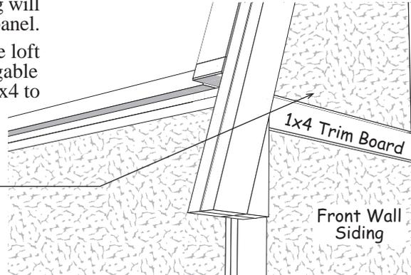
2. Nail bottom edge of siding to 1x4 trim with 6d galv. nails.
