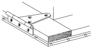
4. Install the left door first. The siding on the left door extends beyond the door frame.
