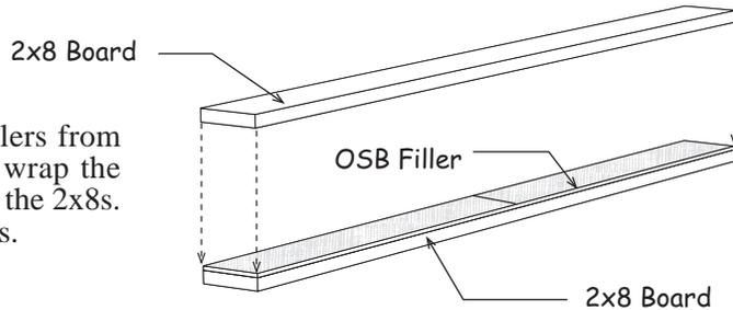
2. Cut (2) two 7-1/2" x 48" long fillers from OSB sheathing that was used to wrap the pallet. Install these fillers between the 2x8s. Assemble header using 16d sinkers.
