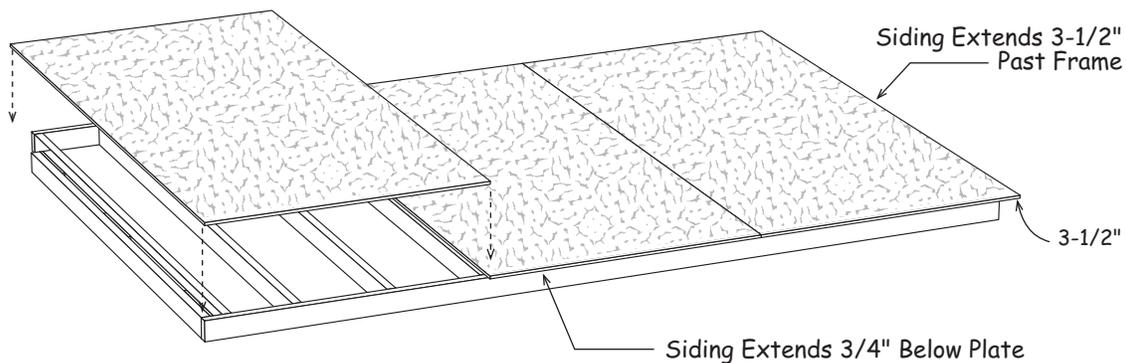
6. Install (2) two full width siding panels.
