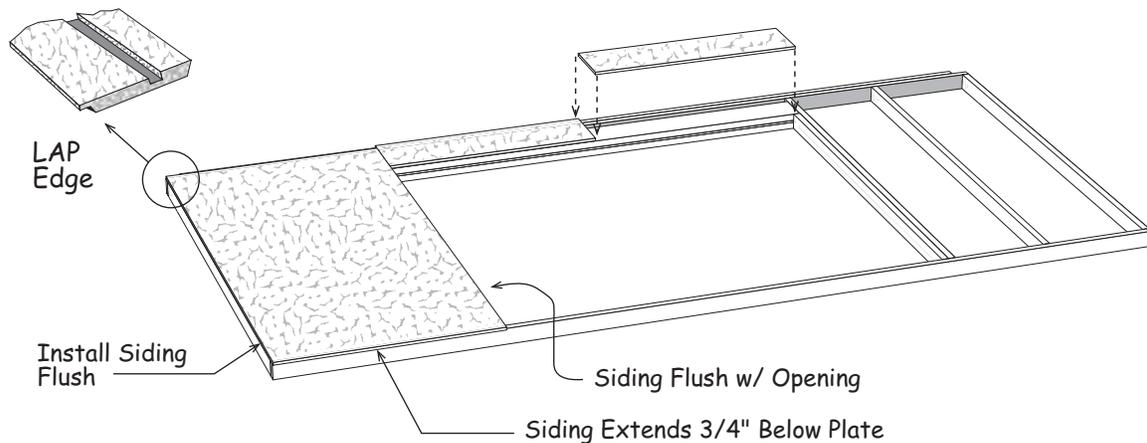
9. Install the pre-cut 12" high siding panels above the door opening. Install the siding extending 3/4" below the bottom of the door header.
