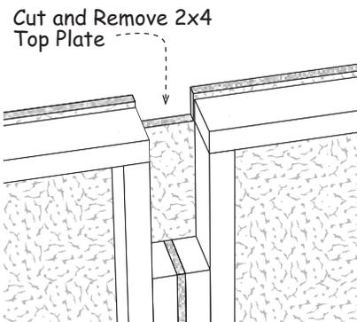
5. Cut the 2x4 top plate. Cut through the siding to remove the 2x4. The siding does not have to be removed. The soffit, when installed later, will cover the cut marks in the siding.
