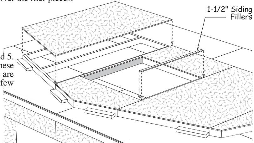
3. Locate gable panels 4 and 5. Remove the siding from these panels. The siding panels are tacked to the walls with a few nails.
