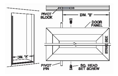
Insert a nylon pivot bushing [M] into the bottom pivot bracket [D]. Slip the second pivot bushing over the top pivot pin on the door panel. Position the door by inserting the bottom pivot pin into the bottom pivot bracket. Hold the door vertical and slide the top pivot bracket into the pivot bushing. Secure the top pivot bracket with a #6 x 3/8" truss head screw [E] and a #8-32 x 1/8" Allen set screw [F].
