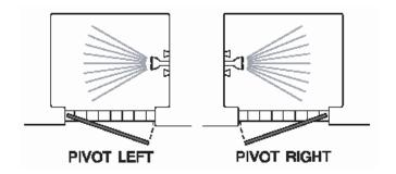
Note: This enclosure may be installed without using the sloped curb [A] provided. Its use is definitely recommended for positive water control on shower sills with little or no slope.
