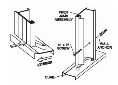
Replace the pivot jamb and attach to the wall with three #8 x 2" truss head screws [J].
