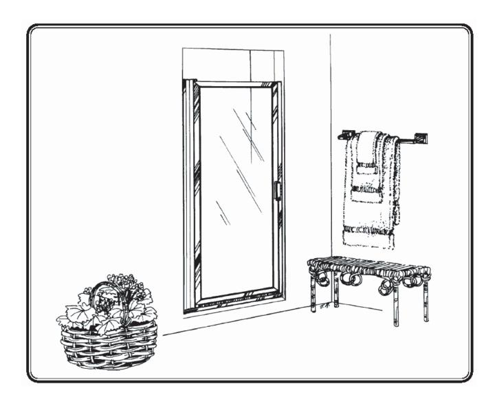
**MAINTENANCE:** Two primary materials are used to manufacture your new bath enclosure: tempered glass and anodized aluminum. To assure a long lasting finish on the enclosure, wipe it down with a towel after each use. Never use a scouring agent to clean the aluminum.
