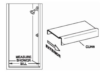
Run two beads of caulk inside the penciled marks on the shower sill. Place the curb [A] in the exact position marked in Step #2 and seat it firmly in the caulking. Also caulk the ends of the curb to the walls. Hold curb into place with masking tape.
