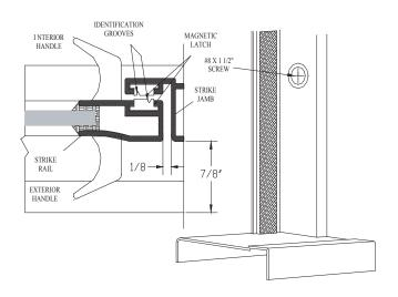
Attach the interior door handle [R] and the exterior door handle [S] to the door with two #6-32 x 1 1/4" round head screws [T].
