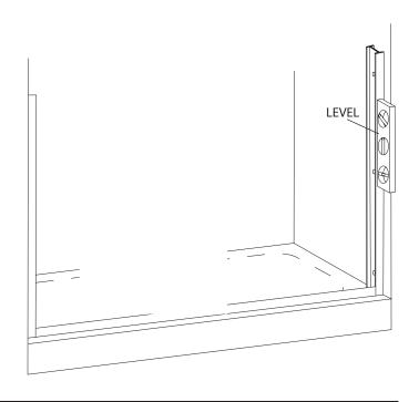
Before replacing the tub track [A], force a slight downward bow in the extrusion. This will ensure the track fits tight to the tub. Run two beads of caulk inside the penciled marks on the tub rim. Place the tub track in the exact position marked in Step #2 and seat it firmly in the caulking.
