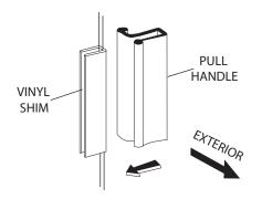
Before installing the door panels, the proper orientation should be determined. For maximum water-proofing, the interior panel should always be positioned closest to the shower head, as shown in this illustration.
