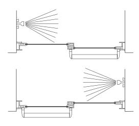
Lift the interior glass panel into position with the rollers engaging the groove in the header [F]. Repeat for the exterior panel. If panels are not parallel to their respective wall jambs, remove and adjust the rollers up or down in their slots to compensate.
