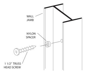
This bath enclosure is equipped with safety teelock wall jambs. When installed properly, the header is permanently locked to the wall jambs and cannot be accidentally dislodged.
