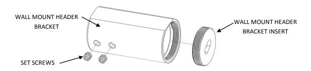
Next, put the supplied large wall plugs into the hole. Screw the inner part of the Header Bracket into the wall with the supplied socket countersunk head screw.
