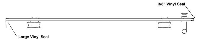
17 The larger vinyl seal will need to be cut slightly in order for the header bar to have space to roll freely. See example below.
