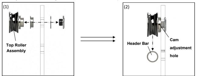
13 Install the bottom rollers as shown in example 1. Adjust the bottom rollers so that they are centered vertically with the top rollers. (see example 2. Bottom rollers may not make full contact with the header bar). Tighten all fasteners to secure position of rollers.
