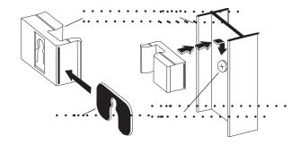
Neatly caulk each end of the tub track [A] where it meets the wall jambs [B] and the interior edge of the wall jambs as shown. Run a bead of caulking along the interior edge of the tub track.
