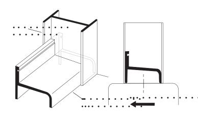
Use a level to plumb both wall jambs [B], then mark the pre-drilled hole locations on the wall. Lightly mark along both sides of the tub track [A] with a pencil, then remove all parts.
