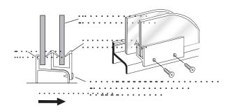
Slide the stainless steel bumper inserts [U] into the four soft vinyl jamb bumpers [V]. Align the slots in the bumpers with the glass panels and snap the bumpers downward over the top and bottom wall jamb screws [D] with the spacers [E].
