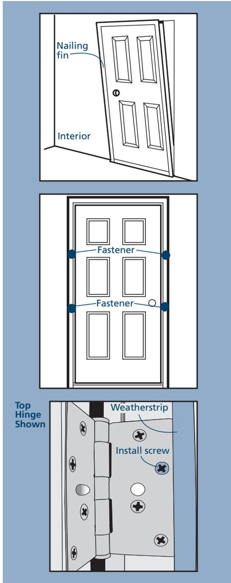
4. Install one of the provided #9 x 2 1/2" screws in the top hinge through the open hole as shown, driving it through the hinge jamb and into the studs.
