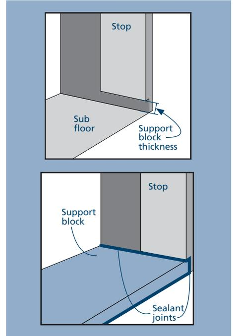
3. Cover the support block and any exposed subfloor with liquid applied flashing or self adhesive flashing. If using self adhesive flashing that requires multiple pieces, begin from the exterior and work in, overlapping the previous piece (shiplap method). Run a bead of sealant on both ends where the blocking material meets the jambs.
