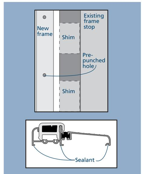
2. On the bottom of the replacement threshold, apply a full length bead of sealant to each leg or measure the locations and mark the existing opening sill. Apply a continuous 3/8" bead of sealant to each line.
