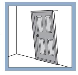
3. Temporarily fasten the door as follows. For metal frames, drive a nail or screw through one lower hole in the flange. For doors without a sidelite(s), secure the hinge jamb by placing one 10d casing nail (or one #8 x 2-1/2" deck screw) horizontally centered in the hinge jamb or brickmould trim 20" from the top and bottom (or just above the lower hinge) of the door. Do not set nails/screws. For appearance reasons. fasteners can be driven behind (but
