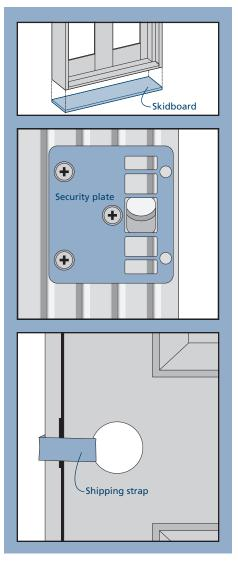
Note! If the door has shipping straps, DO NOT remove them until instructed to do so. These hold the door system aligned and closed during installation.
