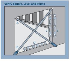
Verify the door is 1" narrower and 3/4" shorter (1/2" each smaller if code requires) than the rough opening width/height. 90-minute fire doors should be 1-1/4" narrower and 5/8" shorter.
