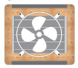
**2. Wide Mount:** The AFG can be mounted on a wide louver, but additional mounting steps must be taken in order for the fan to work properly. As shown in Figure 2.1B, two additional boards must be fastened to the boards framing the gable vent so the AFG can be mounted securely.
