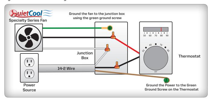
Figure 3.1B: Thermostat Wiring in a Remote Location
