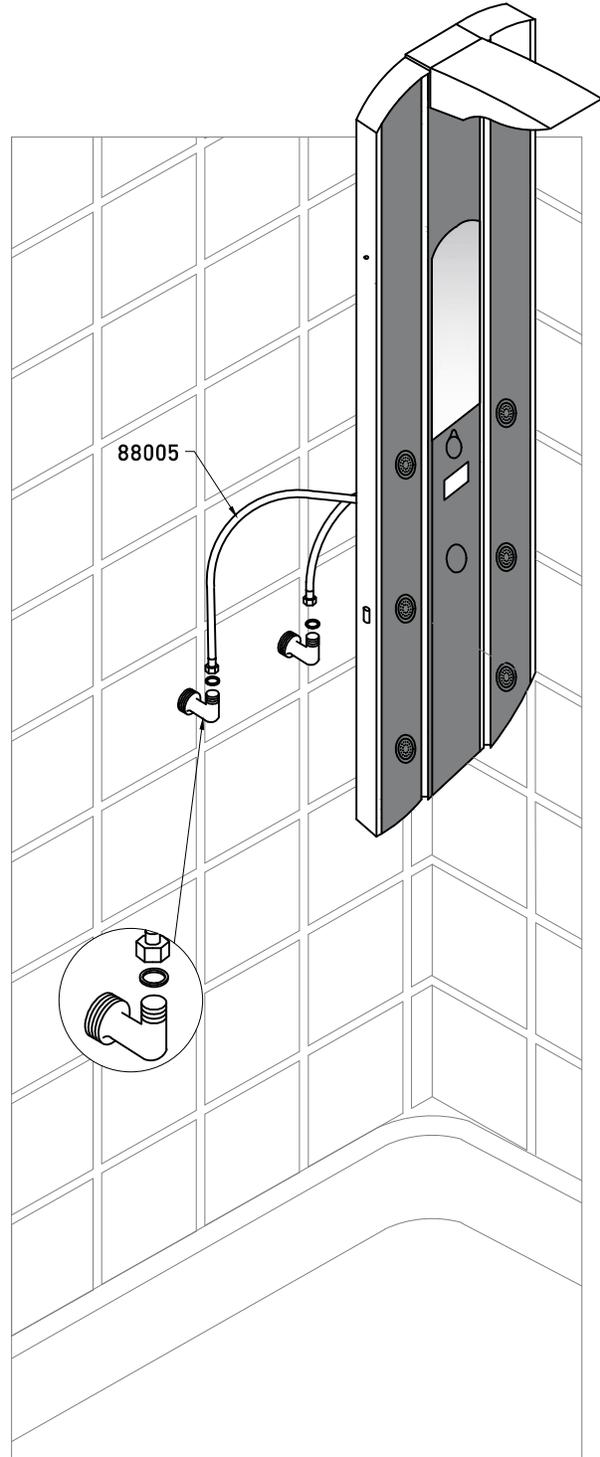
Save time and frustration: if turning the volume/temperature control handle gives both hot and cold water, but the water does not mix, the hoses may have been connected to the incorrect supplies. Please disconnect the hoses, reattach them to the correct supplies and test the unit.
