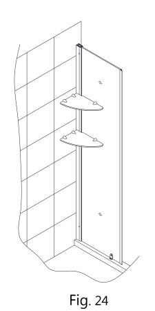
24. Apply silicone sealant between the tray or threshold, the stationary glass and the accessory. Also, apply silicone between the wall and the wall profiles.
