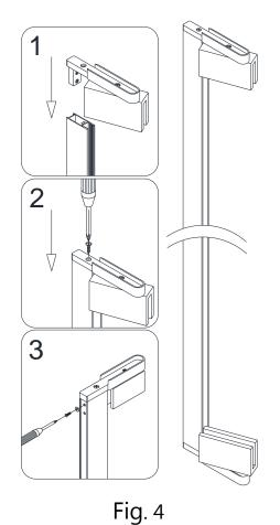
5. Slide the Glass profile for glass door (02) with Pivot assemblies (07) into the groove of the Wall profile for glass door (01) and secure the upper Pivot retainer (08) to the upper Pivot assembly (07) with Round head socket bolt M6×12 (17).
