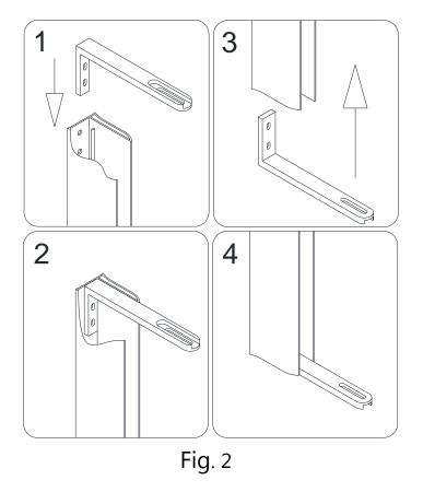
Run a silicone bead along the holes on the wall. Attach the Wall profile for glass door (01) and Pivot retainer (08) to the wall using Round head screws ST4.2×30 (16).
