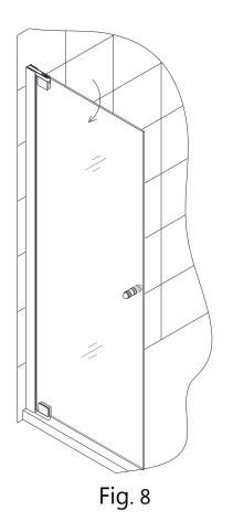
Close the hole in the bottom Pivot retainer (08) with Flat head socket bolt M6×12 (18) or you can attach the Pivot retainer to the Shower base or threshold using Flat head screw ST4.2×30 (16).
