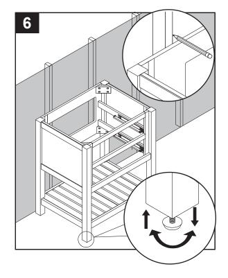
7. Using hardware appropriate for your wall type (not included), secure Vanity Cabinet (A) to two wall studs anywhere through the Vanity Mounting Plates. Be careful not to disturb any electrical or water lines that may be concealed in the wall.
