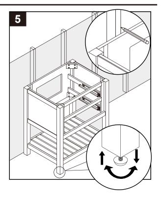
6. Using hardware appropriate for your wall type (not included), secure Vanity Cabinet (A) to two wall studs anywhere through the Vanity Mounting Plates. Be careful not to disturb any electrical or water lines that may be concealed in the wall.
