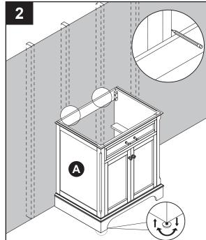
3. Using hardware appropriate for your wall type (not included), secure vanity cabinet (A) to two wall studs anywhere through the vanity mounting plates. Be careful not to disturb any electrical or water lines that may be concealed in the wall.
