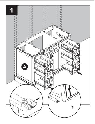
2. Clean area where the vanity (A) will be permanently located prior to beginning installation, ensuring the vanity (A) will not interfere with any water supply and drain lines once mounted.
