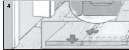
Slide panel into place horizontally and slot in profile. Use these modified planks under doorframes, radiators, cabinet fronts, etc. Use the pull bar to slide the planks where needed.
