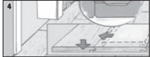
Slide panel into place horizontally and slot in profile. Use these modified planks under doorframes, radiators, cabinet fronts, etc.
