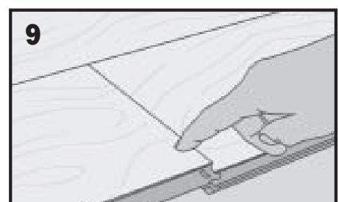
Do not tap end joints with tapping block and hammer. Merely press the end down to lock into place.
