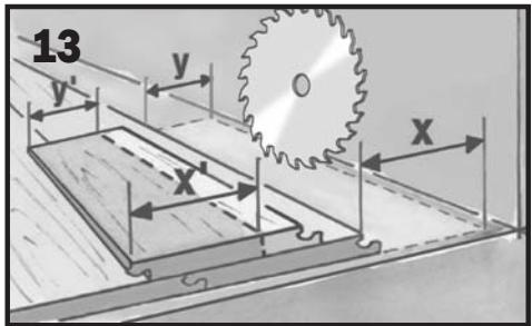
Cut the row along the wall to account for the unevenness of the wall while leaving 3/8 inch expansion room (2.5 inch minimum plank width).
