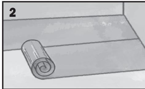
Always use underlayment padding above the vapor barrier and below the laminate flooring planks. If a pad is pre-attached, no additional underlayment should be used.
