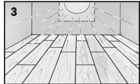
Install flooring parallel to the main light source. If no exterior light source, install parallel to the longest wall.
