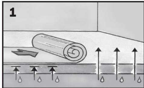
Install vapor barrier if subfloor is cement (6 mil polyethylene film).
