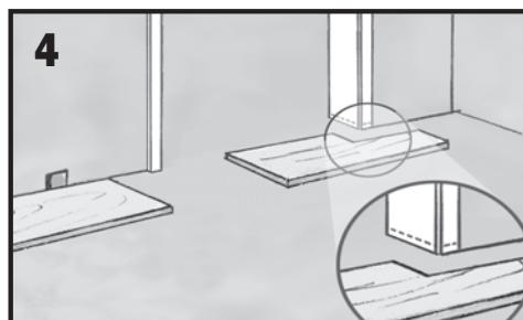
If possible, begin to lay panels under the doorjamb and finish installing planks on a wall without a doorjamb (see working with limited clearance section if needed).
