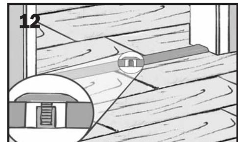
An expansion gap T-strip is required when length of planks measures 40 ft max and when width of planks measures 25 ft max. Transition strips should be placed in all doorways directly under the door when the door is closed.
