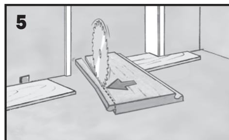
Remove the tongue on the panels adjacent to the walls to allow room for spacers and prevent problems from spills.
