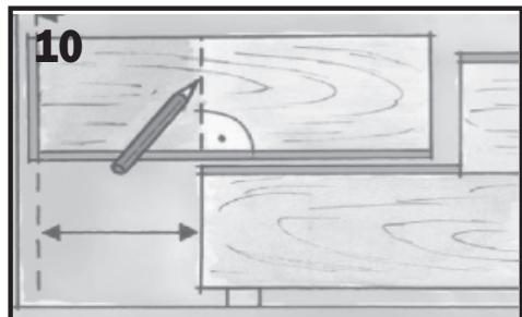
Rotate offcut section 180° and mark accordingly.
