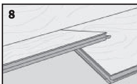
With lengthwise connection made, lower plank into place.
