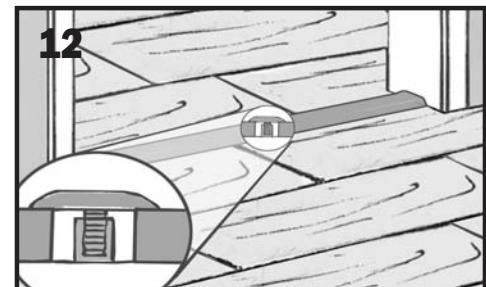
An expansion gap T-strip is required when length of planks measures 40 ft max and when width of planks measures 25 ft max. Transition strips should be placed in all doorways directly under the door when the door is closed.
