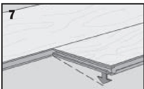
Install planks from right to left as you face the starting wall. Lock in panels lengthwise. Stagger end-joints a minimum 12 inches from row to row.
