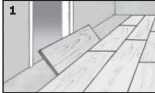
Some long edge joints cannot be installed using a 12° angle.
