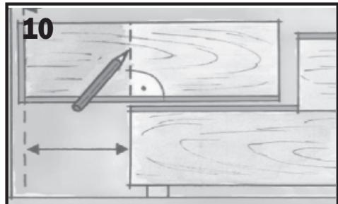
Rotate offcut section 180° and mark accordingly.
