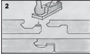
To adjust for this, first remove top part of groove profile.
