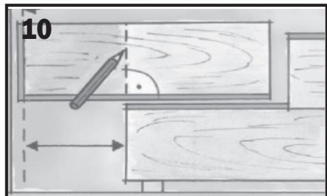
Rotate offcut section 180° and mark accordingly.
