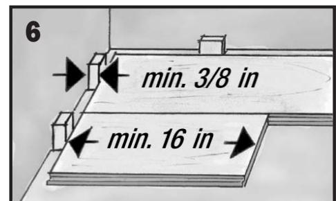
Observe 3/8 inch clearances for expansion and 16 inches minimum for smallest usable piece.
