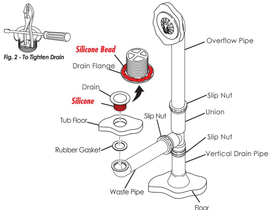
Fig. 1 - Securing Your Drain
