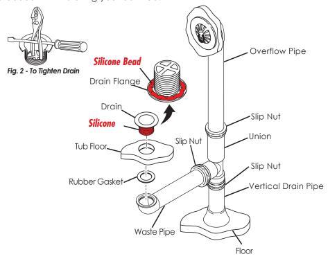
Fig. 1 - Securing Your Drain
