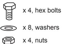
Attach the mailbox to the post using the 4 bolt sets included with the post, as shown below. Be sure to use the washers.
