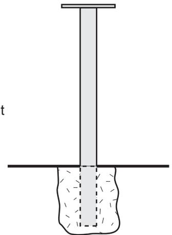
Pour concrete (at least 1 cubic foot recommended) completely around the post. Allow concrete to set before use.
