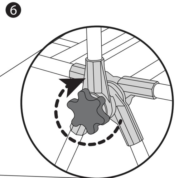
Turn clockwise to tighten securely
