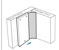
Firmly push Thermostop against Garage Door and fasten. Rubber seal should be in contact with Garage Door, but not not overly tight. Place 2 fasteners within 1/2" of all ends and splices. All other fasteners should be 8" on center entire length of board.
