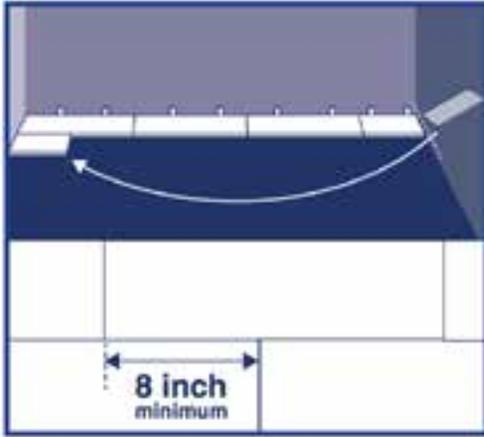
**Step 3:** Use leftover plank from first row as starter for second row. There must be at least 20cm between plank end joints on adjacent rows. **FOR TILE INSTALLATIONS:** The distance between end joints should be
