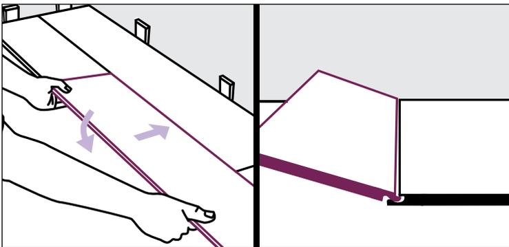
**STEP 10** Tap the length end to ensure a tight fit, then tap the short end to drive down the short end tongue into groove.
