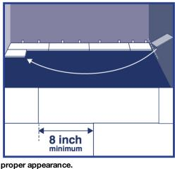
Step 3: Use leftover plank from first row as starter for second row. There must be at least 20cm between plank end joints on adjacent rows. FOR TILE INSTALLATIONS: The distance between end joints should be equal to 30cm for
