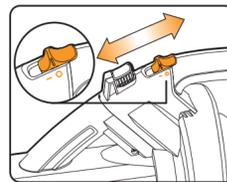
**REMOVING CLOGGED DEBRIS**
