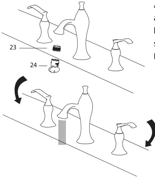
After installing faucet, remove aerator (23) with included aerator key (24). Turn water on for 30 seconds to remove any debris. Reassemble aerator (23)
