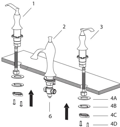
Install faucet body (2), hot handle valve (1), and cold handle valve (3) through 1-3/8" predrilled hole in countertop. Attach rubber washer (4A), metal washer (4B), mounting nut (4C), and mounting screws (4D) on the threaded mounting pipe. Tighten mounting nut (4C) until snug. Tighten screws (4D) on mounting nut (4C) with Phillips head screwdriver until snug. Attach three-way connector (6) to faucet body (2).
