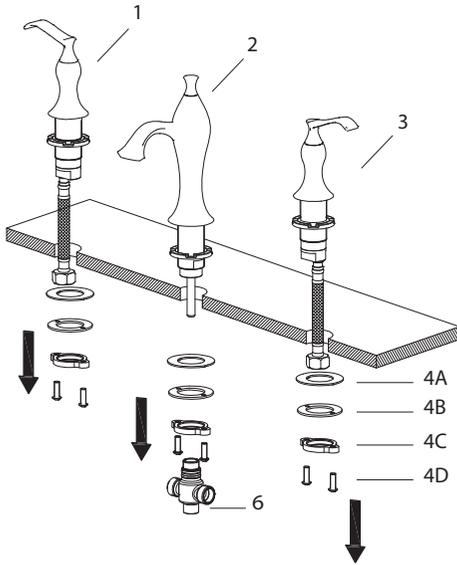
Remove three-way connector (6) from faucet body (2). Remove mounting screws (4D), mounting nut (4C), metal washer (4B), and rubber washer (4A) from faucet body (2), hot handle valve (1), and cold handle valve (3).
