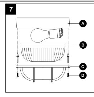
• Note: Before use, add silicone glass sealant between the ceiling and the canopy to completely cover the gap.
