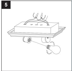
6. Remove knob (H), cap (G), nut (F), rubber ring (D) and washer (C) from the threaded nipple (B). Tighten the threaded nipple (B) into the fixture (A). Place the washer (C), rubber ring (D), and glass shade (E) onto the threaded nipple (B). Tighten with nut (F) and place the cap (G) onto the threaded nipple (B). Tighten with knob (H).
