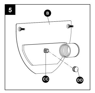
Install light bulb (not included). Use 60-watt max. standard-base incandescent bulb or halogen/ CFL/LED equivalent.
