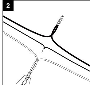
3. Attach wire nuts (AA). Tape wire nuts (AA) and wires together.
