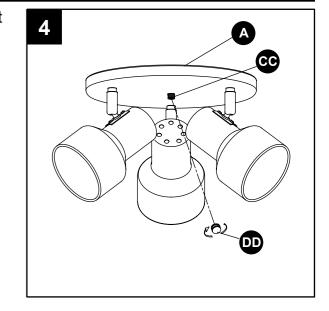
5. Install light bulbs (not included). Use three 60-watt max. standard-base bulbs or three 13-watt standard-base CFL bulbs.
