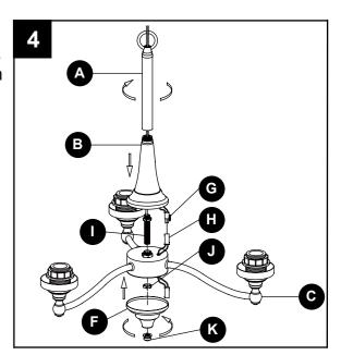
Choose desired installation method, with all of the sockets of fixture (C) facing either upward or downward. Insert plug (G) from decoration (B) into slot (H) of fixture (C), then secure fixture (C) onto the threaded nipple (I) using the hex nut (J), cover (F) and knob (K).
