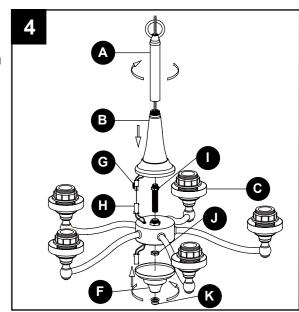
5. Choose desired installation method, with all of the sockets of fixture (C) facing either upward or downward. Insert plug (G) from decoration (B) into slot (H) of fixture (C), then secure fixture (C) onto the threaded nipple (I) using the hex nut (J), cover (F) and knob (K).
