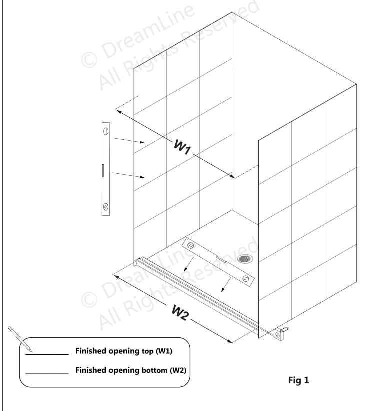
**2.** Cut the **Upper Guide Rail (#01)** and the **Bottom Rail (#08)** to fit your finished opening using either a miter saw or a hacksaw:
