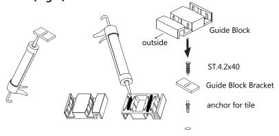
**TIP:** Use one of the Guide Block Brackets as an 1/8" spacer to offset the bracket's placement from the wall
