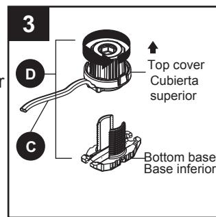
4. Insert wire from low-voltage transformer (sold separately) into the bottom base of connector (D) and then re-tighten the top cover removed in step 3 until the contact pins completely pierce the plastic shield of the wire.
