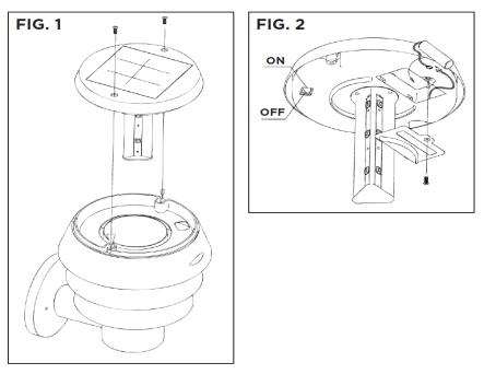
3. Reattach the top (A) to the fixture (B) and secure with the 2 screws.
