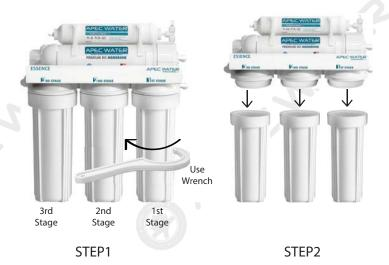
After taking the housing off, take out the dirty filters and put the new 3 pre-filters in. Remember, Stage 2 and Stage 3 are the same carbon filters.
