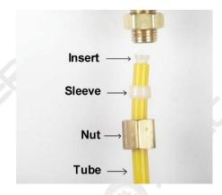
Important! Use <u>plastic sleeve</u> on the plastic tubing we provide. <u>Do Not</u> use metal sleeve on plastic tubing or the connection will leak!
