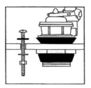
b. Install 2 bolts as follows: Slide rubber washer under bolt head and insert bolt through tank. Install brass washer, then thread hex nut onto bolt. Carefully tighten bolt until snug. DO NOT OVERTIGHTEN or tank may crack.
