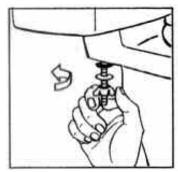
d. Install rubber washer, brass washer, and wing nut onto bolt. Repeat for the other side. Tighten nuts evenly. **DO NOT OVERTIGHTEN** or tank may crack.
