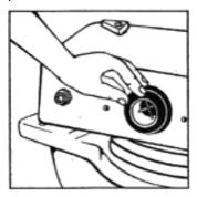
a. Slide new sponge rubber gasket (small side down) onto threaded end of flush valve.
