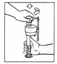
DIAGRAM 3: Replace TOP by engaging lugs and rotating 1/8 turn clockwise. MAKE CERTAIN TIP IS TURNED TO THE LOCKED POSITION. VALVE MAY NOT TURN ON IF TOP IS NOT FULLY TURNED TO THE LOCKED POSITION.
