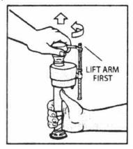
DIAGRAM 1: IMPORTANT: Always clear sand and rust from system. Make sure water supply is off. Remove valve TOP by lifting arm and rotating top and arm 1/8 turn counterclockwise, pressing down slightly on cap.
