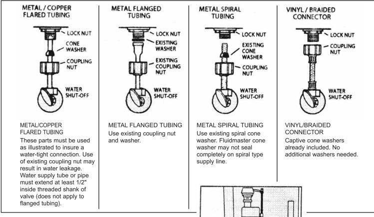
b. With correct washers in place (See previous step), tighten COUPLING NUT 1/4 turn beyond hand tight. DO NOT OVERTIGHTEN.
