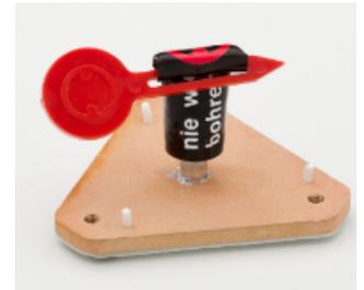
10. Allow adhesive to cure for a minimum of 24 hours. Remove the excess adhesive with a razor knife. **Make sure that the excess from the center hole is removed evenly.** The adapter's surface has to be completely smooth in order to mount the grab bar flush.
