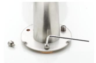
12. Slide cover ring over mounting flange. Turn in one direction until the ring is properly aligned and assure a snug fit. Note there should be a small gap between cover ring and wall to provide proper drainage of water. Note: the cover ring is easily attached if it is turned to the proper position and then snapped on.
