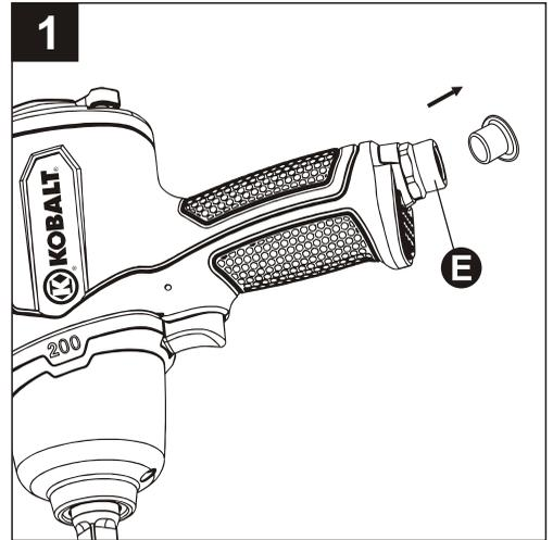
2. Mount a male plug (not included) by hand into the air inlet (E). (See Figure 2)
