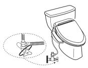
Uphold the appliance and thoroughly drain the water by unscrewing the drain bolt. (beware of losing the drain bolt)
