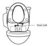
Screw the drain bolt and install the appliance.
