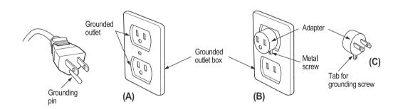
4. If it is necessary to use an extension cord, use only a three wire extension cord that has a three-blade grounding plug, and a three-slot receptacle that will accept the plug on the product. Replace or repair a damaged cord.
