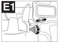
TIP: Always test the spray pattern on scrap cardboard or similar material first. Begin with the material adjustment knob on the highest flow setting (threaded all the way in). If less flow is desired, dial the material adjustment knob out. Heavier, thicker materials should be sprayed with the knob dialed farther in. Thinner materials should be sprayed with the knob dialed farther out.
