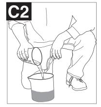
• It is possible to spray latex paint with this unit, however, the required thinning may exceed material manufacturer's recommendation. Thin latex paint so that it runs through viscosity cup in under 2 minutes. The operator should consider the type of application and final location of the project when spraying a material that requires more than 2 minutes to run through the viscosity cup,
