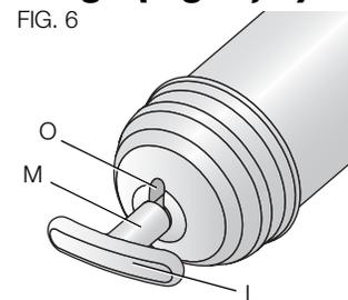
4. Remove the seal from the other end of the grease cartridge.
