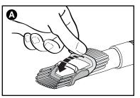
To remove an accessory, press the accessory clip and remove the accessory as shown in figure B.
