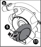
• Tap the back end of appliance if debris does not fall out easily or remove filters for better access.
