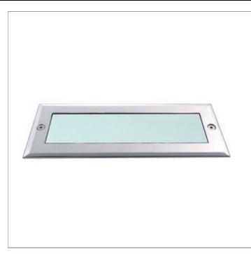
Rectangular MR11 dual up-light. 12V input, remote transformer required, sold separately. Tempered safety glass lens. Stainless steel outer trim. Cast aluminum metal body with powder coat finish. PVC mounting housing included.
