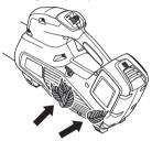
Check that the air intake is not blocked on all sides including the underside, for example, by leaves or rubbish. A clogged air intake reduces the machine's blowing capacity and increases the engine's working temperature, which can result in engine failure. Stop the engine and remove the object. Regularly check that the battery charger and the battery are intact.
