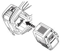
Press on the lower part of the battery and push it in as far as it will go into the battery compartment. The battery will lock itself into place when you hear a click. Make sure the latches snap in place properly.
