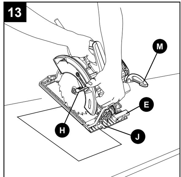
**▲ WARNING:** Always cut in a forward direction when pocket cutting. Cutting in the reverse direction could cause the saw to climb up on the workpiece and kick back toward the operator.
