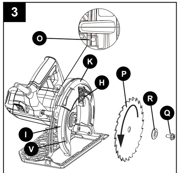
5. Use the blade guard lever (H) to retract the lower blade guard (I) into the upper blade guard (K). Make sure that the lower guard works properly and allows the guard to move freely.
