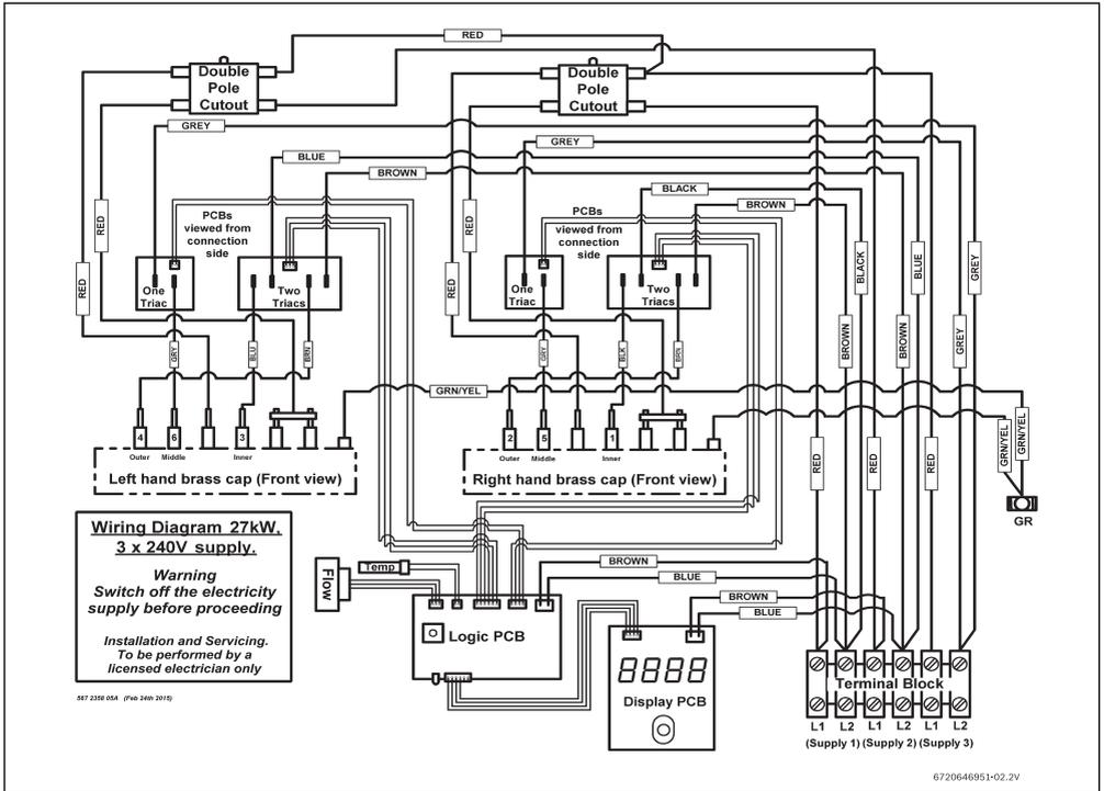
Fig. 4 Internal wiring schematic for single phase WH27 unit.
